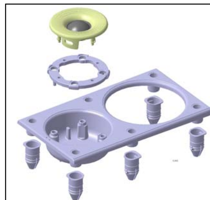
Exploded view of the Decoupled Tweeter Technology.
